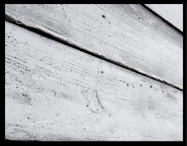
There is +-2mm variation in thickness. There are small differences regarding the length and the width up to 0.5% and it is not considered to be a deficiency or a defect of production, in accordance with the provisions of the conformity with the following standard: EN 492: 2012
