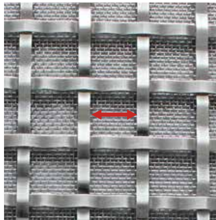
Aperture sizes are measured internally on either the square or diamond patterns.
